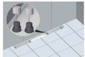
Place the adjusting screws in metal sash.
