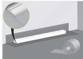
Apply priming coat to leveling concrete. Adhere the isolation tape to the metal-concrete.
