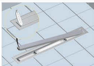
Remove the cover with the help of switch according to your use frequency and then clean it.
