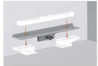
Place the insulation-finish metal case to the adjusting set.
