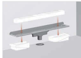
Make a hole from the inside of channel to fix height adjusting sets.
